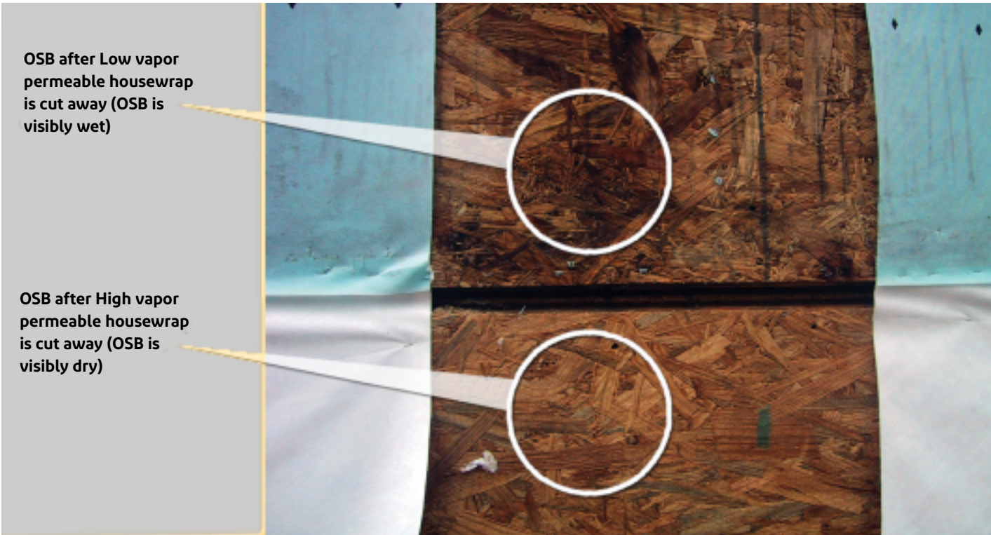
Figure H – Figures F, G & H depict typical findings on the North Carolina wall system during the summer 2002 field investigation. A moisture meter was used to measure the moisture content. Figure F shows the high moisture content behind the low vapor permeability housewrap (moisture meter reading was 27.6). Figure G shows the low moisture content behind the high vapor permeability housewrap (DuPont™ Tyvek®) in an area that was directly below figure F (moisture meter reading was 12.1 – less than half of the reading directly above it.) Figure H shows the condition of the OSB directly behind this transition area.
