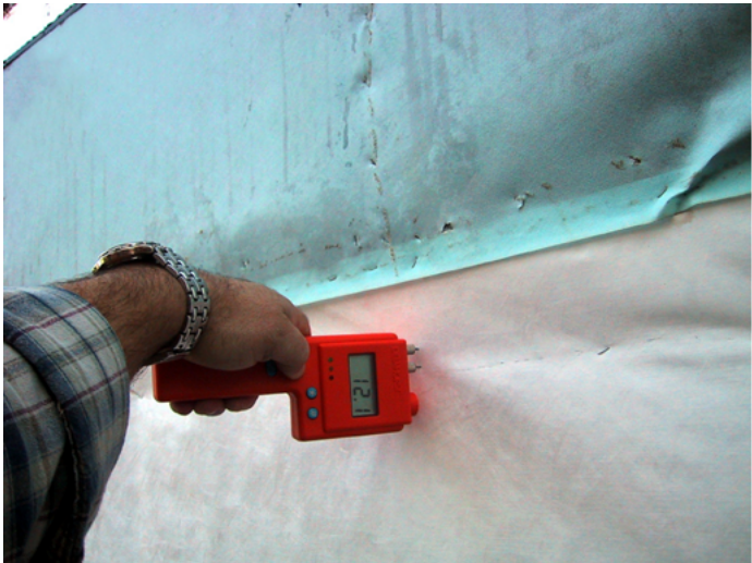
Figure G – High vapor permeable housewrap with low moisture reading on OSB under the DuPont™ Tyvek® HomeWrap®
