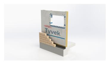
Typical brick cavity wall assembly.
