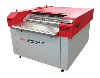
The Cyrel® FAST 1001 TD delivers outstanding plate quality and uniformity. This processor has the ability to produce a finished plate without solvent washout. The wide format Cyrel® 1000 ECLF for exposing the light-finishing plates is available to complement the Cyrel® FAST 1001 TD as an all-round system solution. As with all elements of the Cyrel® FAST system, it is environmentally friendly with no solvents to handle, store or recycle and no drying equipment is required.
