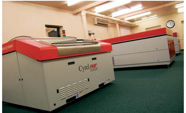
**With the installation of the new Cyrel® FAST Promopack became the first UK Platemaking business (serving the wide web flexo market) to completely eliminate solvent from the manufacturing process. This meant fewer lorry journeys, better working conditions and ending the need for special waste disposal. It also eliminated all fugitive (solvent) emissions to atmosphere.**
