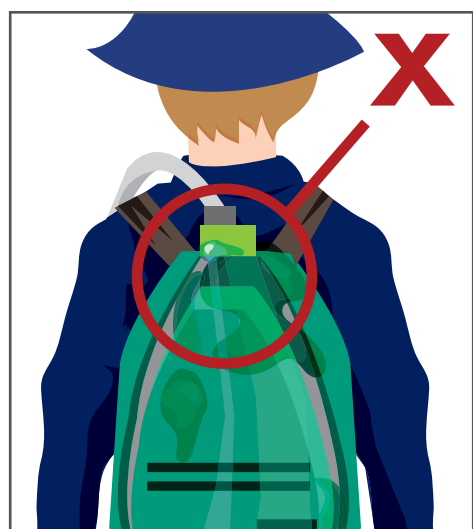
3. DO NOT use the application equipment if it is leaky or damaged. Always check to ensure that the application equipment is in proper working condition.
