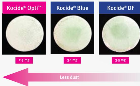
Figure 8: A 30 g sample is allowed to fall under standard conditions in a chamber releasing dust. Dust is collected on filter paper placed on a glass sided filter box. The filter paper is re-weighed and the difference in weights is defined as the “collected dust”.
